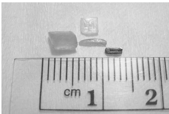
Figure 3. Some representative samples from the IPNS. Although a minimum sample size of approximately 1 \text{ mm}^3 in volume is required for the typical single crystal experiment, in practice larger samples are often desirable.
